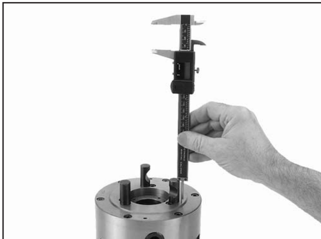
Figure 19. Measuring height of cam-lock studs.
